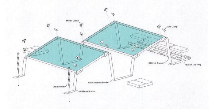
NOTE: The position of the attachment points are calculated by Aerocompact and must be strictly installed according to the static report to be code compliant.
